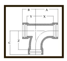
A = Grooved N = Face-Fed BT = SB x SB x NPT(F) RT = SB x NPT(F) x SB BRT = SB x NPT(F) x NPT(F)
